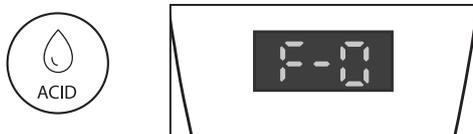
3. On the ECAIA ionizer S faucet, press and hold the "Power (D-D1)" and "Alkaline levels (ALK) (D-D2)" buttons at the same time until the display switches off. This saves the setting.
